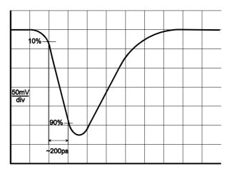
The rise time of the output pulse is related to the rise time of the input pulse and the rise time of the pre-amplifier approximately by the formula :-
