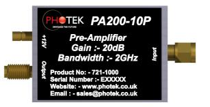
approximately twice their length i.e. a 1ns pulse input will be a 2ns pulse output. The amplification ratio is a minimum of 20db, i.e. gain of 10.
